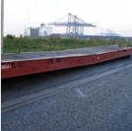
There must be a load on the gooseneck to prevent the roll trailer from tipping backwards.
