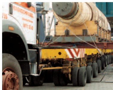
Trailer on the RORO ramp (weight approximately 360 metric tons). One 35 metric ton capacity FLT pulling, one heavy ballasted, 4-axle truck pushing & steering.
