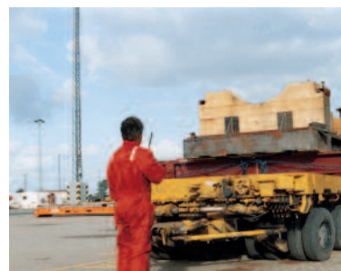
12-axle, 96 wheeled, hydraulic trailer negotiates the cargo bridges.
