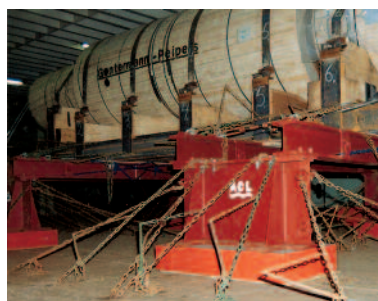
Cargo lashed down for its voyage. Lashing details: Roll to deck: 8 heavy duty lashings; skid to deck: 8 chains/binders; skid to cargo bridges: 8 heavy duty lashings, 28 chains/binders; cargo bridges to deck: 48 chains/binders.
