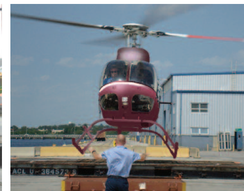
Working with the helicopter's crew member, ACL's specialist carefully guides the craft onto the heli-mafi for a secure landing.
