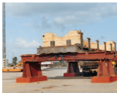
Skid on cargo bridges. The bridges are spaced 4.3 m (14' 1") for proper support of cargo skid and transfer of weight onto two transversals and longitudinals aboard the ship.
